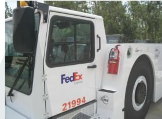
Fender Mounted Fire Extinguishers
